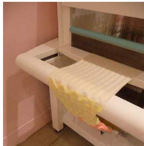
Fig. 1. 3-D woven piece on TC-2 loom, Philippa Brock, 2013 (retroreflectiv and elastic yarns), “Future is Here: A New Industrial Revolution” exhibition [3]
